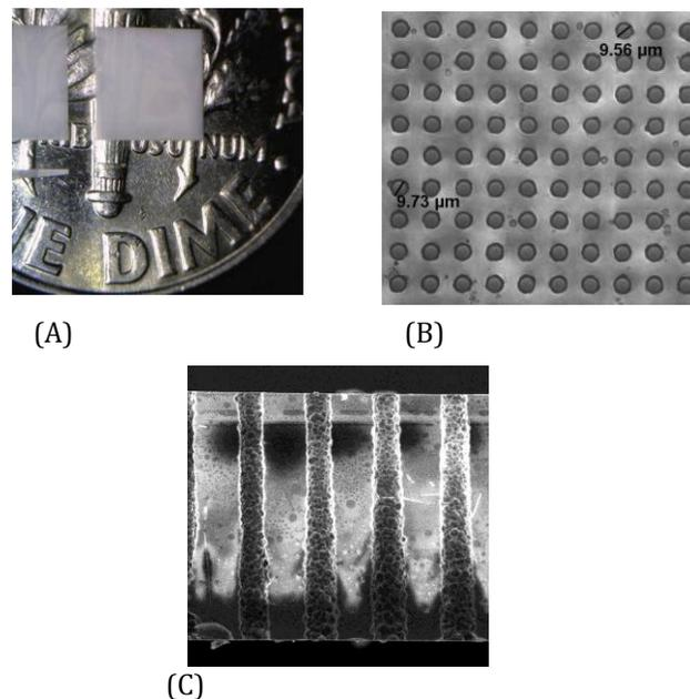
Fig. 4. (A) An array of 40,000 10 micron diameter TGVs on a dime, (B) a close up of 10 micron diameter, 20 micron pitch, TGVs, and (C) a SEM image of the 10 micron diameter TGV cross section.
