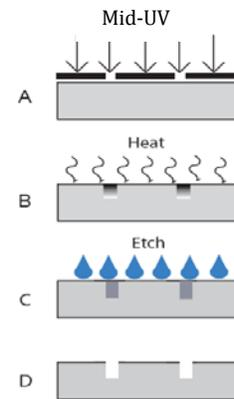
Fig. 1. Processing steps of APEX<sup>™</sup> Glass Ceramic.
