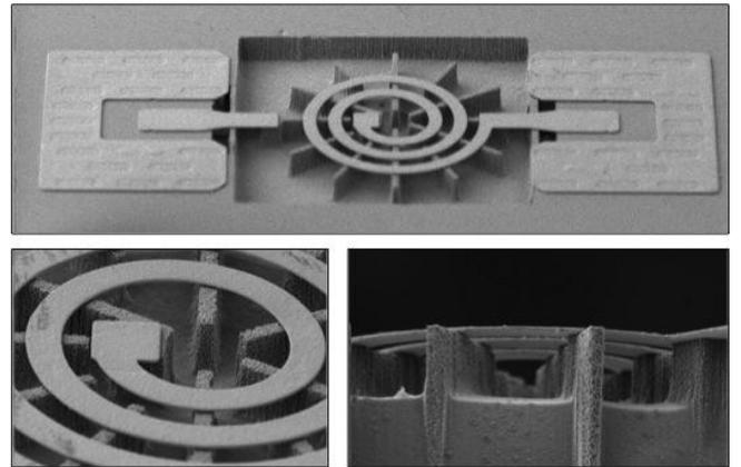
Fig. 3. (Top) Laser ablation of 25 micron diameter TGVs in borosilicate glass. (Bottom) 14 micron diameter TGVs wet etched into APEX™ Glass. Notice the glass sputtering and irregular shape of the ablated TGVs compared to the lack of debris sputtering and the high fidelity of the wet etched APEX™ Glass TGVs.
