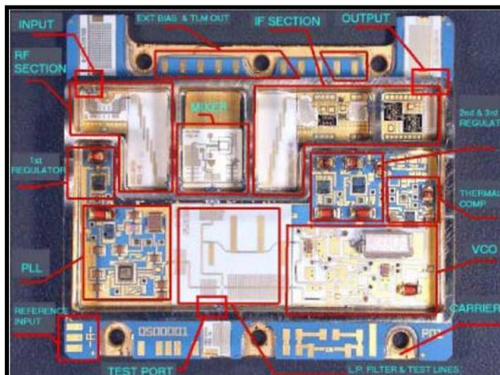
*Figure 3- System in a Package (SIP)*
